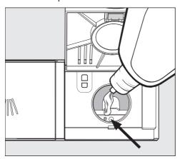
Only add rinse aid until the fill level indicator (see arrow) turns dark when the door is open horizontally.
