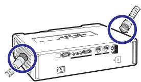
• If you want to clean the air vents during projector operation, ensure you press **STANDBY/ON** on the projector or **STANDBY** on the remote control and put the projector into standby mode. After the cooling fan has stopped, clean the vents.
