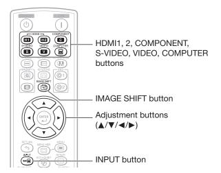
Press ▲/▼/◄/▶ to adjust the vertical and horizontal position of the image.
