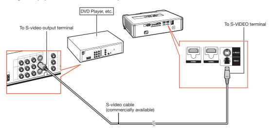
Refer to "Samples of Cables for Connection" on page 19 for connecting other equipment.
