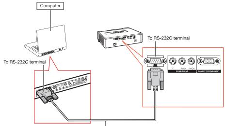
RS-232C serial control cable (cross type, commercially available)
