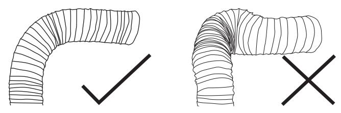
For the Isodrive motor, please do not crush or kink flexi ducting, as it will reduce air flow and may cause noise to occur through the system. Ducting needs to be kept taut at all times.
