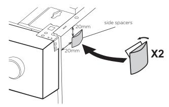
Fit the dishwasher by carefully sliding it into the cavity.
