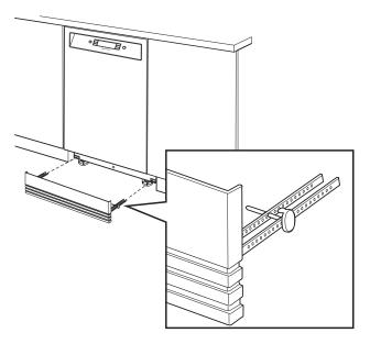
When installing the adjustable plinth to undercounter height cabinets 870-920mm, kit #52075772 must be purchased.
