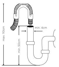
The water drain hose can be connected either directly to the water drain hole or to the sink outlet spigot. Using a special bent pipe (if available), the water can be drained directly into the sink via hooking the bent pipe over the edge of the sink. This connection should be at a minimum of 50cm and at a maximum of 110cm from the floor.
