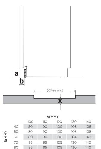
When installing the adjustable plinth to standard undercounter height cabinets (820-870mm), attach the 2 adjusting brackets to the metal plinth with the screws provided.
