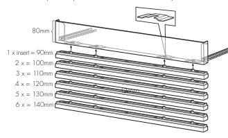
Use the 2 plastic locking pins to set the position of the plinth assembly.
