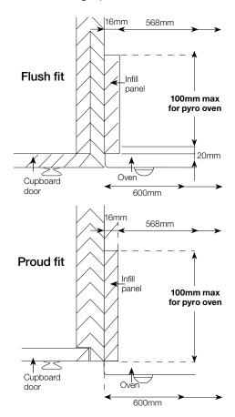
Note: Your appliance must be mounted on a flat surface for the full width and depth of the product
