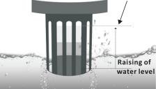
When the tank is full of water, the Protective Device will rise up, suction power will cut off. Pour out all
