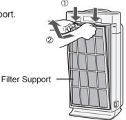
Remove the washable Active Carbon Filter (Black) and HEPA Filter (White) from the plastic bags.
