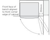
When positioned in a corner area, clearance of at least 350mm on the hinge side will allow the doors to open enough to enable the removal of the bins and shelves. This required clearance inceases to 550mm for those models with telescopic extension slide-out bins.
