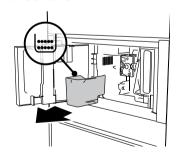
When EMPTY GROUNDS CONTAINER appears on the display, the grounds container must be emptied and cleaned. The appliance cannot be used to again until you have cleaned the grounds container. Even if the container is not full, the empty grounds container message is displayed 72 hours after the first coffee has been prepared. For the 72 hours to be calculated correctly, avoid turning the appliance off from the mains switch if it is not necessary.
