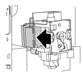
6 After cleaning, replace the infuser by sliding it onto the internal support and pin at the bottom, then push the PUSH symbol fully in until it clicks into place.
