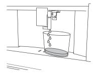
⑦ PLACE 2L CONTAINER UNDER SPOUTS PRESS ✓ TO START DESCALING: Place an empty suitably sized container under the steam wand and coffee spouts.
