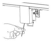
(2) Check that the holes in the coffee spouts are not blocked. If necessary, remove coffee deposits with a toothpick.
