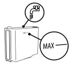
14 RINSE AND FILL WATER TANK UP TO MAX LEVEL: Fill the tank up to the MAX level with fresh water.
