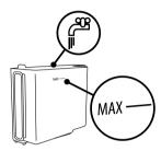
(9) RINSE AND FILL WATER TANK UP TO MAX LEVEL: the appliance is now ready to rinse with fresh water. Empty the container used to collect the descaler solution. Remove the water tank, rinse under running water, fill with fresh water up to the MAX level and put back in the appliance.
