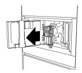
Press the two coloured release buttons inwards and at the same time pull the infuser outwards.
