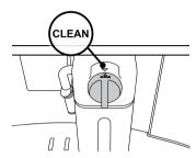
3 Turn the froth adjustment dial to CLEAN, CLEANING MILK CONTAINER UNDERWAY appears on display.
