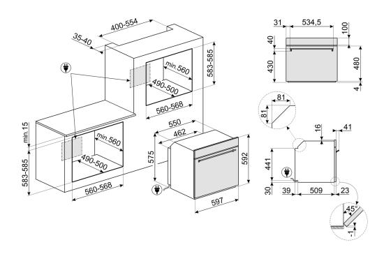
Dimensions  $597 \text{mmW} \times 592 \text{mmH} \times 548 \text{mmD}$
