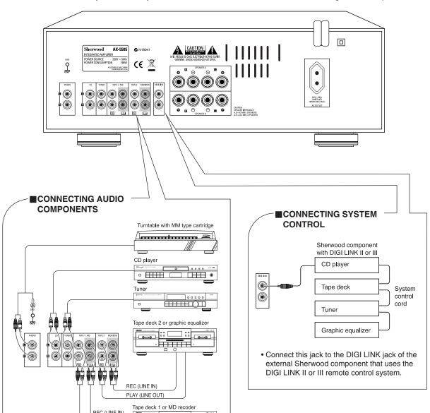
The TAPE1/MD IN/OUT jacks may also be connected to the LINE OUT/IN jacks of an additional MD recorder.
