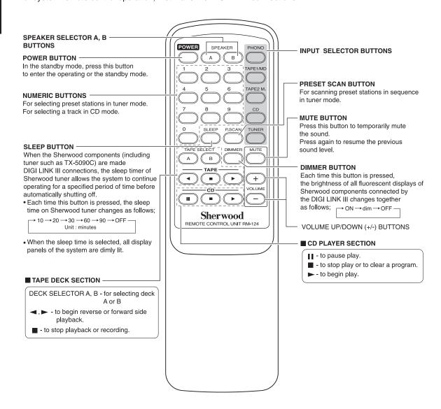
• In the DIGI LINK III remote control system, if pressing PLAY, etc. on CD player or tape deck, CD or TAPE 2 MONITOR is selected automatically without selecting the input source and then PLAY, etc. starts.
