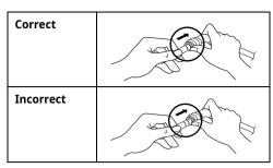
If the water tube end is damaged, it should be trimmed to ensure it does not leak when refitted.
