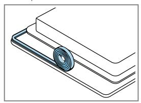
3. Move the shorter part of the adhesive seal strip supplied into the area underneath the front part of the hob. If necessary, cut the adhesive seal to the required length.
