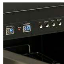
Computerized temperature control
