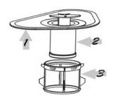
Main filter Food and soil particles trapped by this filter are pulverized by a special jet on the lower spray arm and washed down the drain.
