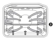
The bottom heater, the round heater, and the hot air fan will operate. Suitable for baking pizzas, apple pies, and fruitcakes.
