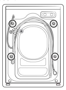
Locate the shipping bolts (marked with circle in the figure) on the rear side of the washing machine.
