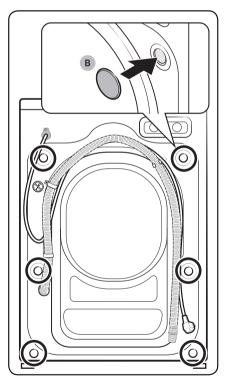
2. Using the supplied spanner, loosen all the shipping bolts by turning them counterclockwise.
