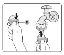
6. While pulling down part (D) on the water hose, connect the water hose to the adaptor. Then, release part (D). The hose fits into the adaptor with a clicking sound.
