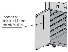
To light manually, unclip match holder and fit a 40mm match to the holder and light. Pass match through viewing slots below the front of the cooking plate down towards the burner, then rotate the control knob to HIGH to ignite. If ignition fails, turn the control valve OFF and allow several minutes for the gas to disperse before attempting to light again.
