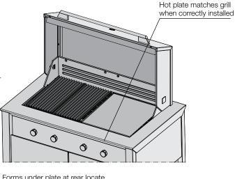
Forms under plate at rear locate on rear of burner box to give slope for grease drainage
