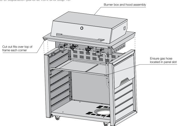
**B.** Once in position, open the hood and align the side burner box formed holes with the side brackets. Fit 2 screws with fibre washer each side.
