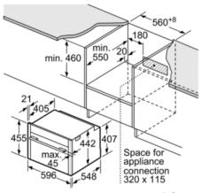
measurements in mm
