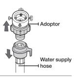
2. First, using a '+' type screwdriver, loosen the four screws on the adaptor. Next, take the adaptor and turn part (2) following the arrow until there is a 5 mm gap.
