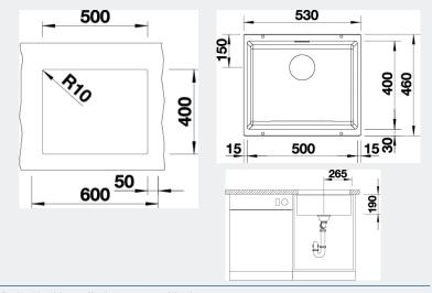
Undermount Method of Installation:
