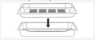
The grid or the tray should always be inserted into the groove between the two wire profiles.
