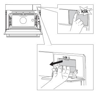
■ Apply pressure to open the water tank door.
