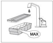
Open the water tank cover and wash it with water. Before use, add fresh water up to the MAX marking on the tank.
