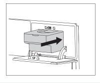
Push the water tank back into the housing to the position in which the position switch is activated. Then, press the tank door to close it.
