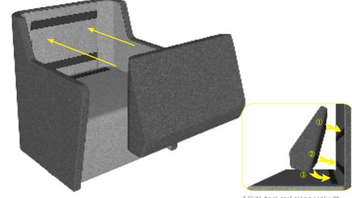
\* Slide back rest along seat with top racked forward to fasten upper velcro set first.
