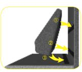
\* Slide back rest along seat with top racked forward to fasten upper velcro set first.
