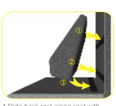
\* Slide back rest along seat with top racked forward to fasten upper velcro set first.
