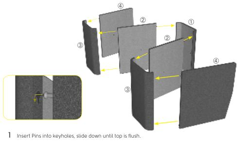
**2** Once panels are flush, slide pin across to lock panels together.
