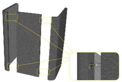
1 Insert Pins into keyholes, slide down until top is flush.
