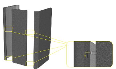
Insert Pins into keyholes, slide down until top is flush, locate the velcro strips on the top of the panels with those on the under of roof panel.
