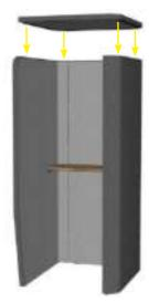
5 Locate th velcro strips on the top of the panels with those on the under of roof panel.
