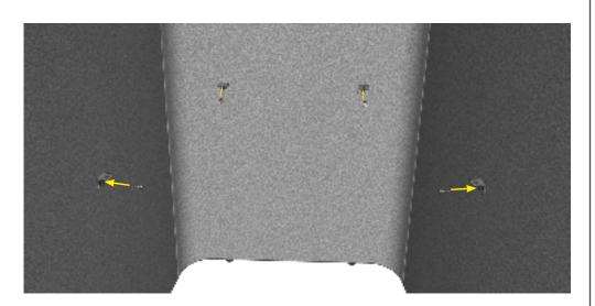
4 Place the worktop onto the fixed brackets, then screw bolt though the bracket in to the T-nut on the underside of the worktop.
