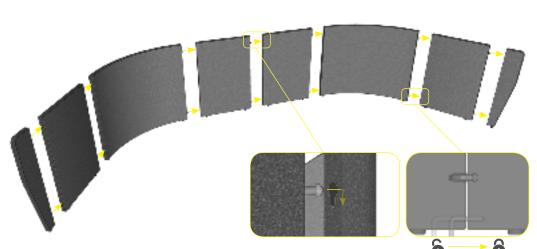
Start with curved panel, insert Pins into keyholes, slide down until top is flush. Once panels are flush, slide pin on the underside of the panel across to lock panels together.
