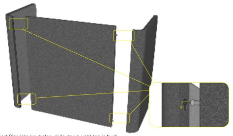
1 Insert Pins into keyholes, slide down until top is flush. **2** Once panels are flush, slide pin across to lock panels together.
