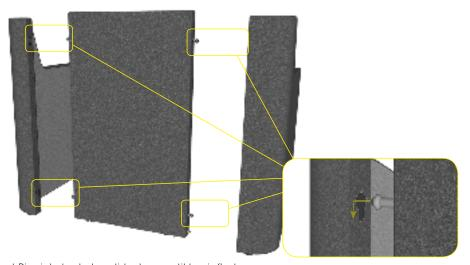
1 Insert Pins into keyholes, slide down until top is flush.
