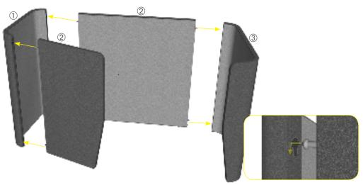
Start with panel 1, add the two panel 2 to 1 then lock them together as shown in Step 2. Continue this until item is assembled completed.
