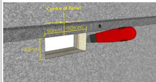
2 Find the centre of the panel, cut away fabric & foam over the lateral cut out. Do this on both sides.
