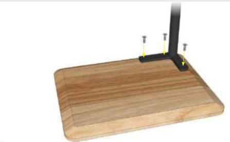
2 Screw bolt though the worktop holder in to the T-nut on the underside of the worktop.
