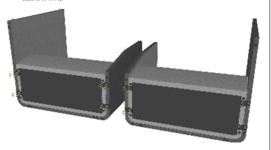
4 Locate the velcro strips on the backrest & the roof with those on the panels.
