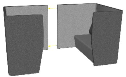
**5** Join the two side panels together as step 1 & 2 above.
