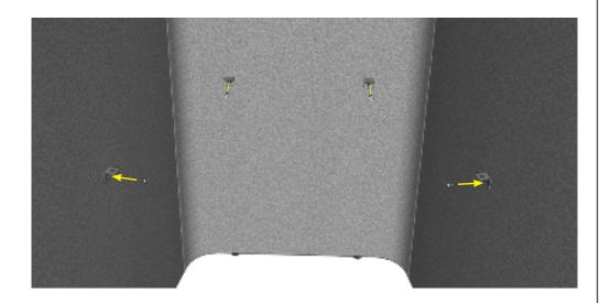
4 Place the worktop onto the fixed brackets, then screw the worktop to the brackets using wood screws.
