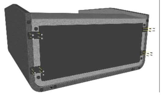
**4** Locate the velcro strips on the backrest & the roof with those on the panels.
