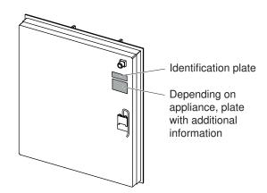
► Affix the second identification plate (supplied) in an accessible position behind the front of the fitted cabinet beneath the appliance.
