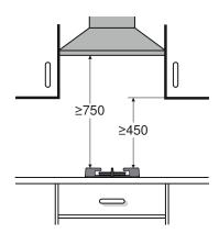
When a range hood is installed above the gas hob, the minimum distance given for the particular range hood must be observed.
