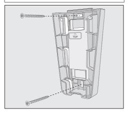
Attach the mounting plate to the wall.
