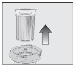
■ Lift the fine dust filter upwards to remove it.
