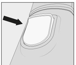
To separate the individual sections from each other, press the release catch on the Electrobrush and pull the connector out of the Electrobrush.
