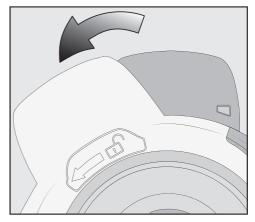
Turn the lid of the dust container in the direction of the arrow as far as the first stop.
