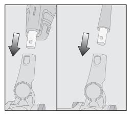
Insert the connector down into the Electrobrush from above until it audibly clicks into place.
