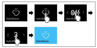
Fig. 47 Example illustration: Activate HydroBreeze with value 3.
