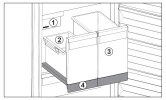
Fig. 99 Pull-out board with IceTower
