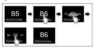
Fig. 26 Example illustration: Switch from B5 to B6. Carry out action steps according to the illustration.
