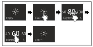
Fig. 56 Example illustration: Switch from 80 % to 60 %.
