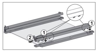
Fig. 121 Glass shelf with rails and retaining parts Install rail with damping mechanism:
