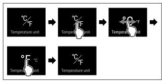
Fig. 21 Example illustration: Switch from degrees Celsius to degrees Fahrenheit.
