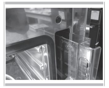
At the end of the procedure, the message DISCHARGE ENDED / REMOVE AND EMPTY THE TANK will appear on the display, confirming that the discharge was successful. If you do not wish to immediately repeat a new steam cooking cycle, it is recommended to empty the container and replace it in its housing, then close the door.
