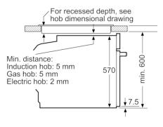
measurements in mm
