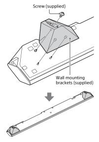
Prepare screws (not supplied) that are suitable for the holes on the rear of the Bar Speaker or surround speakers.
