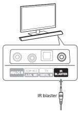
Place the IR blaster close to the remote control sensor of the TV, aiming the IR emitter of the IR blaster at the remote control sensor of the TV.
