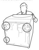
2 Attach the two front brackets to the bottom of the Main Washer and screw up each bracket using machine screws(7 EA).
