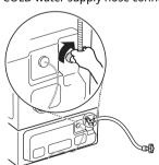
3 Connect one end of the cold water supply hose connector to the cold water supply hose of the Main Washer first.
