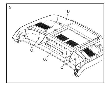
6. IMPORTANT: To avoid damaging the Pulse Crossbar (80), do not use power tools, and do not overtighten the #10 x 3/4" Screws (6) or the 5/16" x 2" Screws (2).
