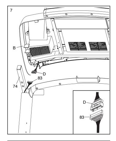
Attach the console assembly (B) to the Handrails (74) with four 5/16" x 2" Screws (2) and four 5/16" Star Washers (8). Start all four Screws, and then tighten them. Be careful not to pinch the wires.
