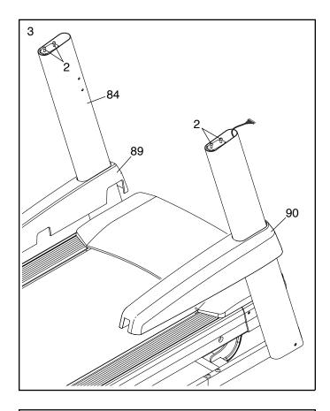
Attach the two Handrails (74) to the Uprights (84) with two of the 5/16" x 2" Screws (2) that you removed in step 3 and two 5/16" Star Washers (8). Do not fully tighten the Screws yet. Be careful not to pinch the Upright Wire (83) on the right side.
