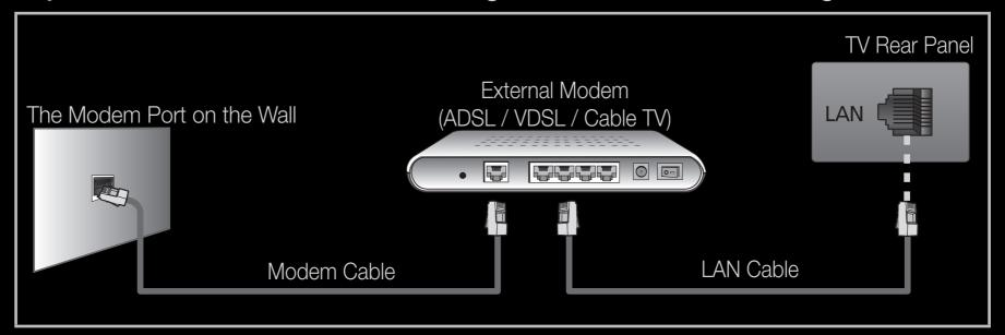
You can attach your TV to your LAN by connecting the LAN port on the back of your TV to a IP Sharer which is connected to an external modem. Use LAN cable for the connection. See the diagram below.
