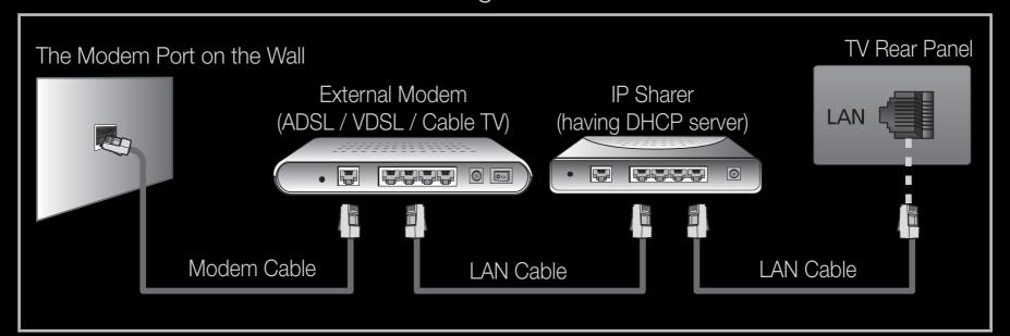
Depending on how your network is configured, you may be able to attach your TV to your LAN by connecting the LAN port on the back of your TV directly to a network wall outlet using a LAN cable. See the diagram below. Note that the wall outlet is attached to a modem or router elsewhere in your house.
