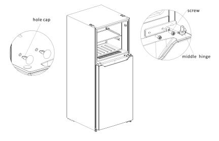
**Step 4** Install the hinge shaft and shaft sleeve to the left hole of the bottom hinge (seen below) to the left corner of the refrigerator, Then adjusting the levelling foot according to the position shown below. Then place the other levelling foot back into place on the other side.
