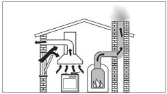
Great care should be taken when using the downdraft extractor at the same time and in the same room or area of the house as another heating appliance which depends on the air in the room. Such appliances include gas, oil, wood or coal-fired boilers and heaters, continuous flow or other water heaters, gas cooktops, or ovens which draw air in from the room and duct exhaust gases out through a chimney or extraction ducting.
