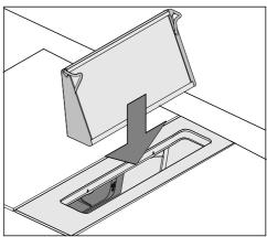
■ Fit the grease filter so that the straight side of the grease filter is on the side that connects to the air duct.
