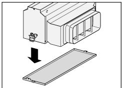
■ Remove the drip tray from the casing.
