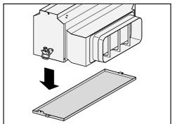
■ Remove the drip tray from the casing.
