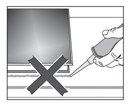
The SmartLine appliance and worktop may be damaged if the appliance needs to be removed after it has been sealed with a sealant. Do not use any sealant between the
