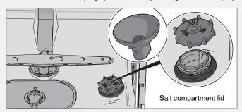
When the salt runs out, unscrew the cap and fill the container with salt. Water is only needed the first time! Wipe clean and tighten. Run a program to ensure that any salt in the dishwasher is rinsed away.
