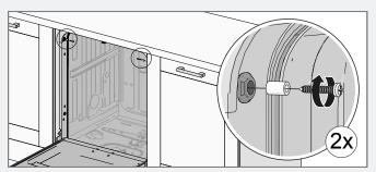
After fastening the machine, check that the front feet still touch the floor.
