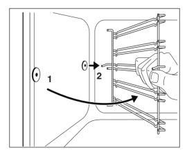
3. Install the rack supports by following the procedure described in reverse order.
