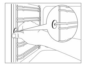
2. Pull out the back of the shelf support from the side wall and remove it.
