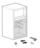
Place refrigerating chamber door on bottom hinge then fix the middle hinge on left side and insert the hole caps on right side;
