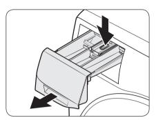
1. While holding down the **release lever** inside the drawer, slide open the drawer.
