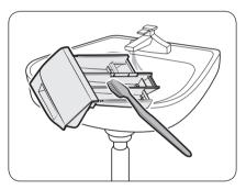
2. Clean the drawer components in flowing water using a soft brush.
