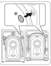
3. Insert the **bolt caps (B)** to the holes (marked with circle in the figure).
