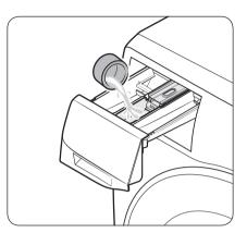
3. Apply fabric softener to the **softener** compartment. Do not exceed the max line.
