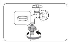
1. Connect the water hose to the water tap, and then turn it to the right to tighten.
