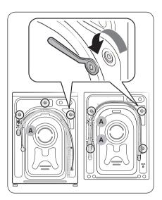
1. Locate the shipping bolts (marked with circle in the figure) on the rear side of the washing machine.
