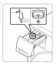
First insert the provided liquid detergent container in the III main-wash compartment. Then, apply liquid detergent to the container below the marked max line (A).
