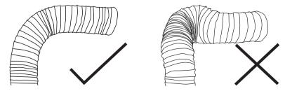
For the Isodrive motor, please do not crush or kink flexi ducting, as it will reduce air flow and may cause noise to occur through the system. Ducting needs to be kept taut at all times. Please refer to the Isodrive motor installation guide for more details on flexi ducting with the silent system.
