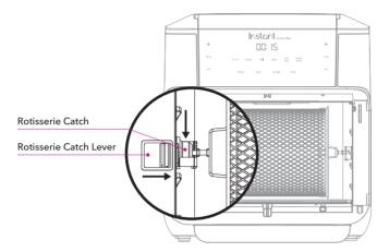
3. Align the left side of the accessory with the hole in the rotisserie catch, and set the right end of the accessory in the notch on the right.
