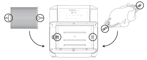
Move the red rotisserie catch lever to the right and hold it in position. Notice that the rotisserie catch inside the cooking chamber withdraws slightly when you move the lever.
