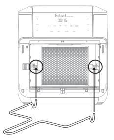
3. Move the rotisserie catch lever to the right and hold it in position to release the accessory.
