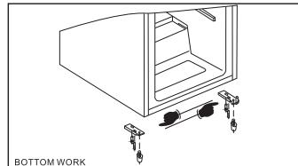
Unscrew the upper pin and screw it into place on the opposite side.
