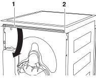
► Take the tower panel 1 out of its fixture 2 on the back of the tumble dryer.
