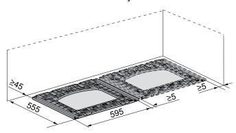
In order to keep the distance to the wall, fold out the spacers D on the installation plate.
