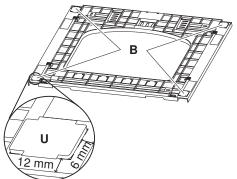
▶ Adhere the mounts **U** to the mounting surfaces **B** precisely.
