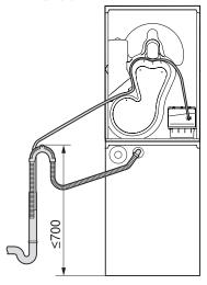
Drainage into fixed upright outflow pipe with combi drainage set (W55969):
