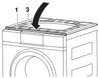
▶ Install the tower panel 1 on the mounted installation plate 3.
