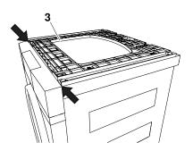
► Turn over the installation plate 3. Push to the front edge of the washing machine cover plate (see arrow) and adhere into place.
