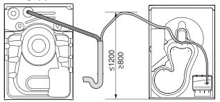
Drainage into fixed upright outflow pipe with combi drainage set (W55969):
