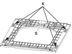
► Take out the double-sided adhesive tape **S** and adhere to the mounting surfaces **K**.
