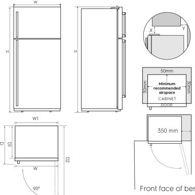
If you have a cupboard above the refrigerator with a rear gap of less than 100mm (Y), recommended minimum clearance at the top of the refigerator increases from 30mm to 70mm (X).
