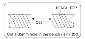
Pass all the hoses, tubes and USB lead through the 35mm hole.
