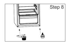
9. Remove the hinge bushing and door stop of the R-door and F-door with screw driver, and install them to the other side of the doors.
