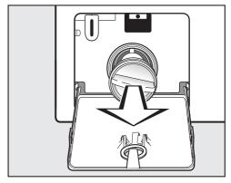
■ Remove the drain filter completely.
