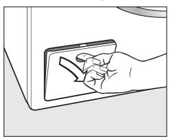
■ Open the drain pump access panel.
