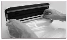
Close the lid, press and hold pressure on the middle of the lid to start the vacuum sealing. The LED light should turn blue to indicate that the vacuum sealer is under vacuum.
