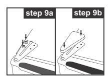
10. Once the door is in place and all bolts (top hinge bracket and bottom hinge bracket) are securely tightened, insert caps on right side of the freezer and door.
