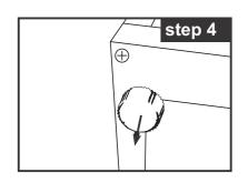
5. Fasten the bracket to the left side of the freezer. Do not tighten completely to enable slight adjustments to the door once in place. Fasten the adjustable foot.
