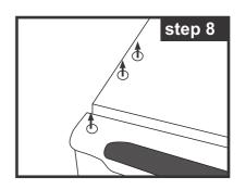
9. Place the hinge on the left side and align the holes before screwing in bolts. Do not tighten bolts completely until after aligning the door and ensuring proper seal between the door and the freezer. Replace the hinge cover.
