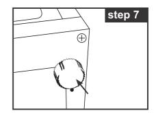
8. Remove the caps covering the bolt holes and door from the left top side. Place the door onto the bottom hinge pin.
