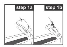
2. Lift the door from the hinge. Place the door in a safe location to avoid scratches or damage.
