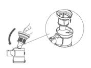
8) Assemble the top cover to the dust cup.
