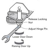
(3) After adjusting door height, firmly tighten the Locking nut ( ) counter-clockwise until secured.
